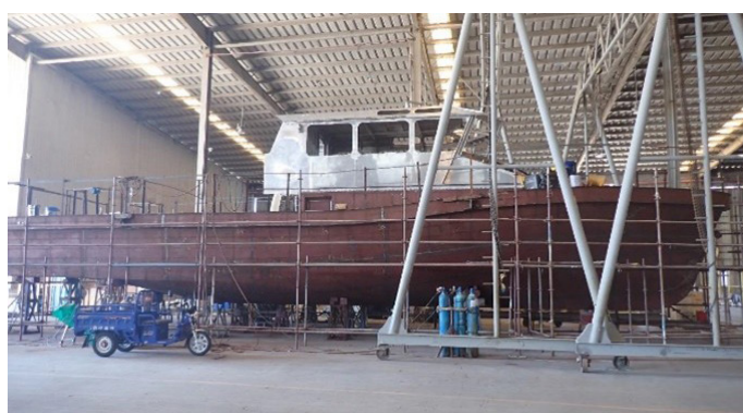
Photo: Manufacturing process of the pilot boat at the shipyard. @UNDP
